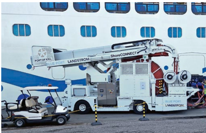
The really big sockets. The AIDANova connected to onshore electric power on 26 August 2023 before putting out to sea from Kiel. Photo: Felix Kolbeck
