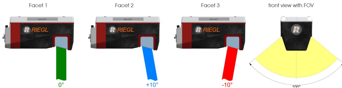
Fig. 3: RIEGL VUX-16023 scan pattern with nadir/forward/backward views
