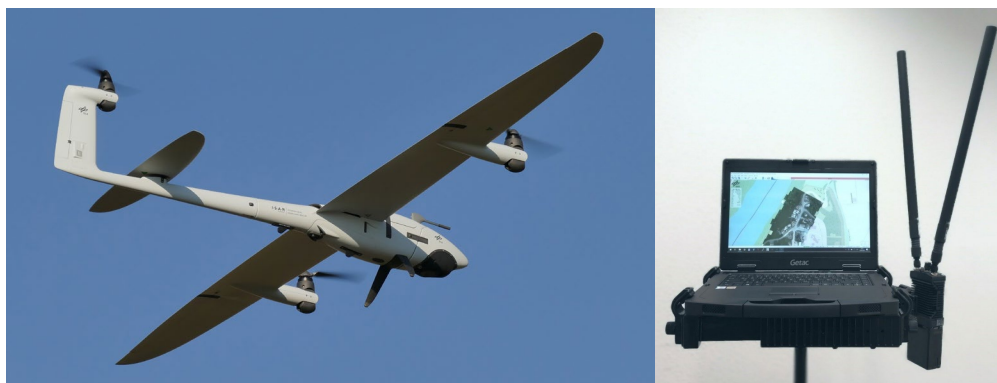
Fig. 3: VTOL drone Vector with latest MACS payload (left) and notebook with radio link module (right) to receive and visualize the situational picture (Source: DLR)
