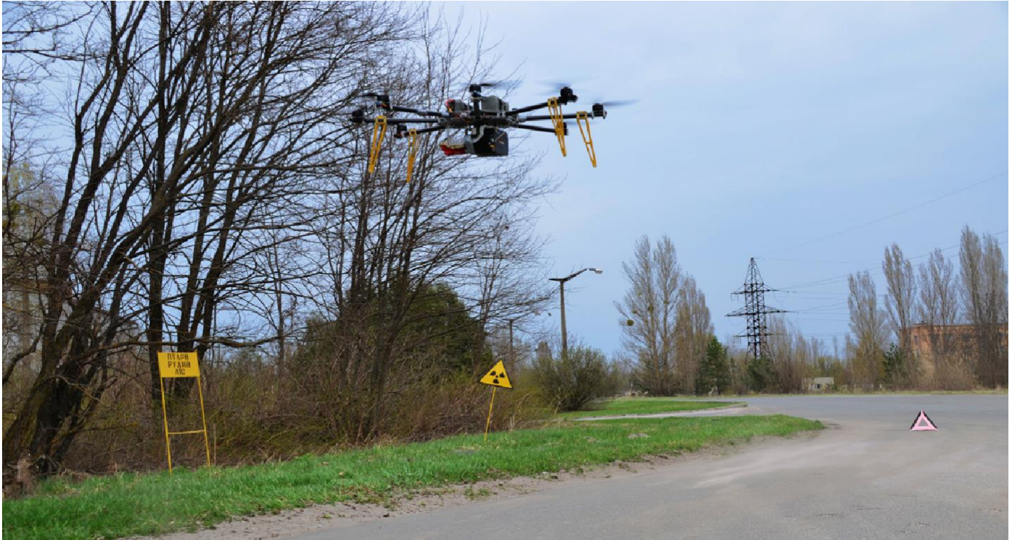
Octocopter with laser scanner and multispectral camera (Illustration: Norbert Molitor)
